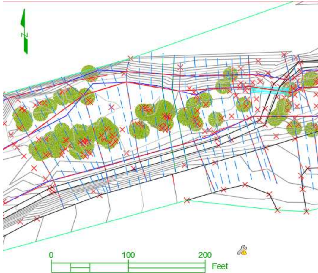
Figure 2-2 - AutoCAD Drawing of Site 1 showing trees and low points within the site.
